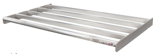
Laterals are constructed of 11/4" x 11/4" x .070" thick tubing. Front lateral is 11/4" x 11/2" x .080"
