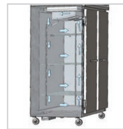
Modular refrigeration air flow
