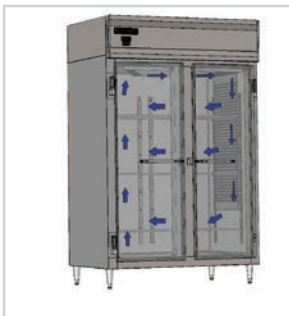
Top and side air distribution ducts
